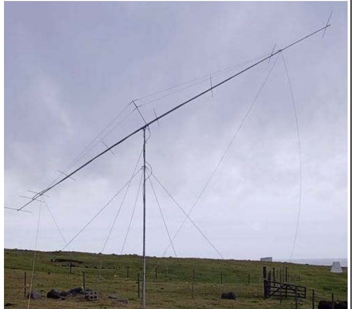
Lance's aerial set up to aim VHF signals at the moon
