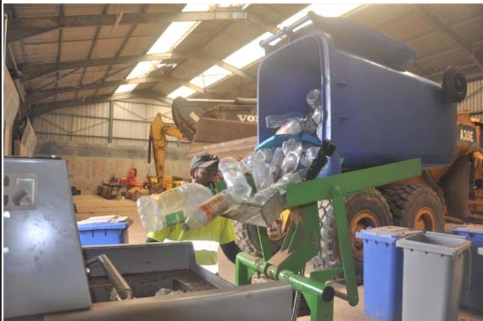
Plastic being loaded into the crusher
