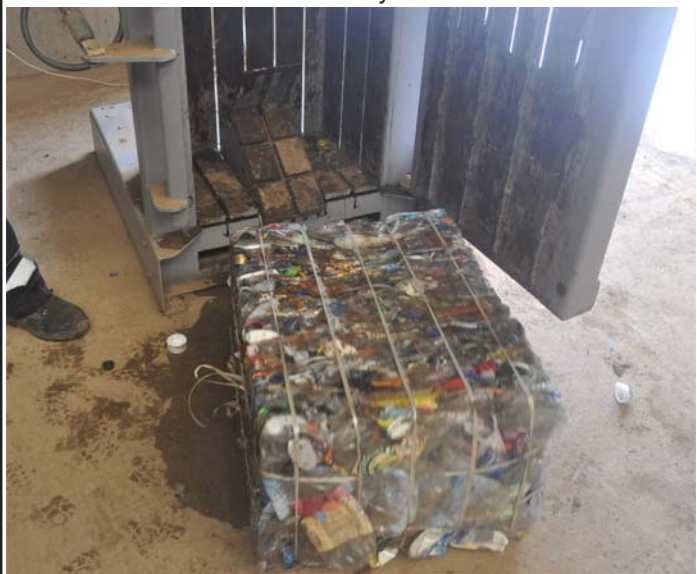
Crushed and baled cans delivered from the crusher
