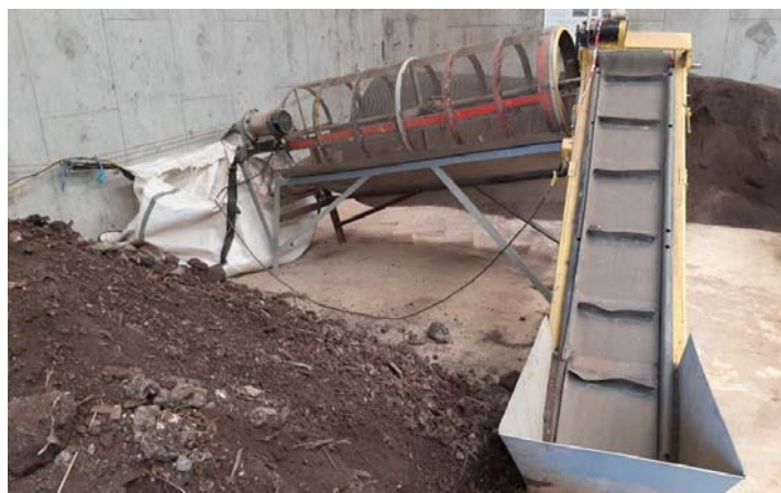
Patrick's compost machines made from waste materials
